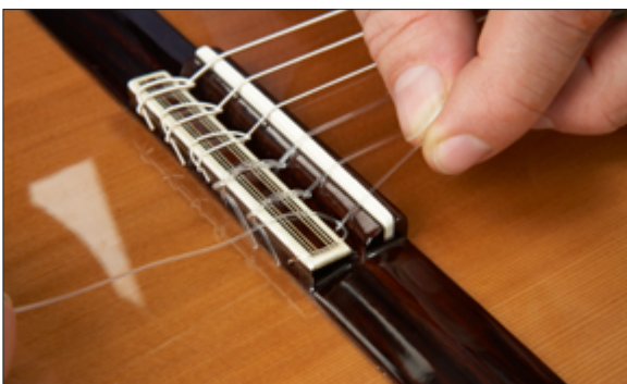
Bridge First Loop
